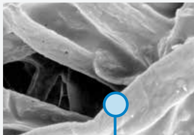
10 Micron Cellulose Media (600x)
